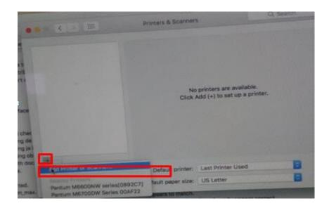
**Step4:** Please choose the corresponding model from installed printer when pop up the dialog box. Then chose the corresponding printer's driver which installed on PC. (It is needed to be the same with printer model.) After chose to save, it will be finished to install.
