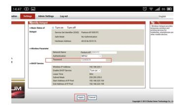
**Step8:** Disconnect equipment and printer, when reconnect them, it should input the password as step 7 setting.
