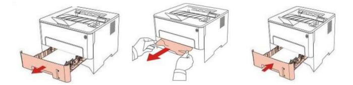
Step2: Open the front cover, take the laser toner cartridge out along the track, then gently pull the jammed paper out.
