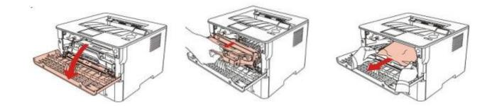
**Step3:** After taking out papers jammed, install the laser toner cartridge again and close the front cover, then the printer will recover printing.
