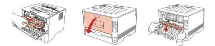
**Step2:** Gently pull the jammed paper out, then c lose the back cover after removing the paper jammed, install a new toner cartridge and then close the front cover; then, the printer will recover printing automatically.
